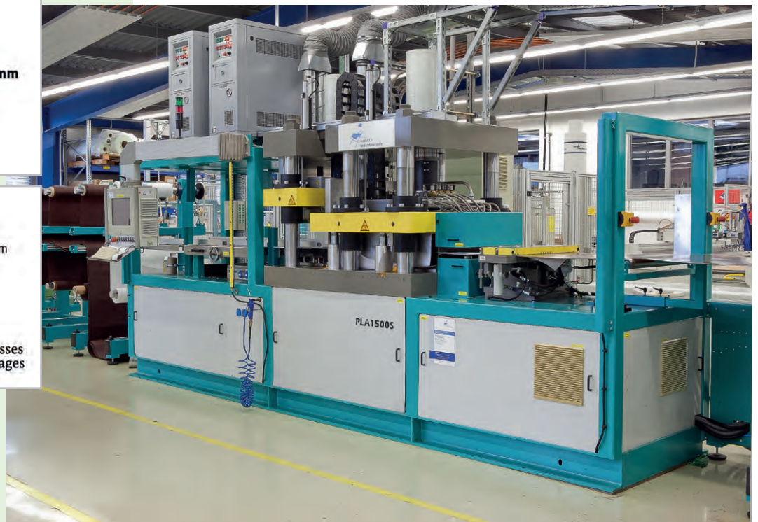
Intervallheißpresse des IVW Semi-continuous compression molding machine of IVW
