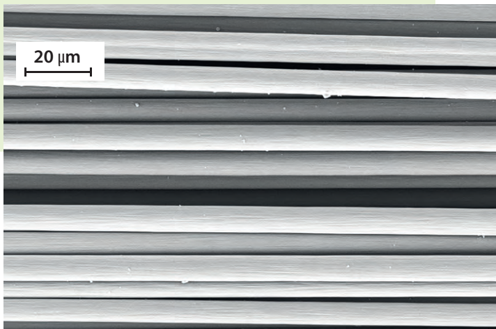
SEM image of a CFRP sample after an optimized thermolysis
